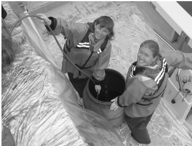
Karen Hudson and Missy Southworth transfer rhodamine dye onto a VIMS research vessel in preparation for a dye release experiment on the York River. The dye will help show how tidal currents might disperse oyster larvae.
