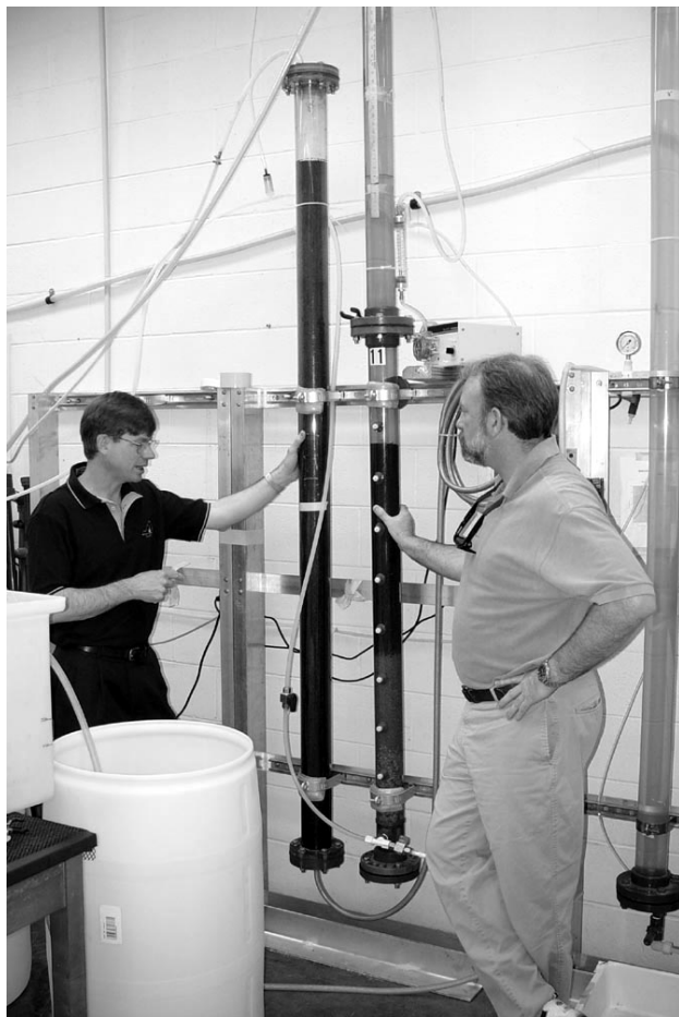
Drs. Gary Schafran (L) and Mike Unger inspect columns of activated carbon like those used to remove TBT from shipyard wastewaters.
