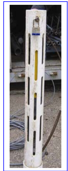
Figure 3.5 Guard-pipe by The Province of British Columbia
