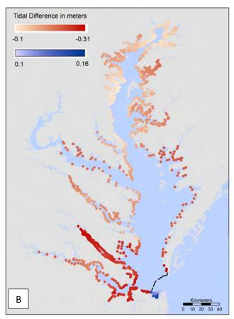
The hydrodynamic model generated tidal ranges for current conditions (Figure A) and the closure scenario. The hypothetical storm surge barrier is shown as the black line across the Bay mouth. Currently, the highest tidal ranges occur at the mouth of the Bay and in the upper reaches of the lower Bay tributaries (e.g. James and York Rivers). Lowest ranges occur along the main stem of the Bay.
