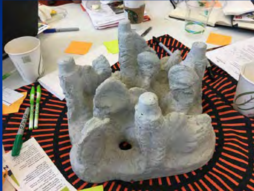
Concrete Oyster Reef Restoration Tile from Grow Oyster Reefs, LLC
