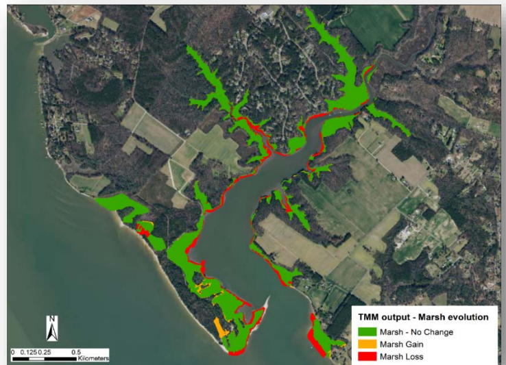
Marsh boundary evolution for Carter Creek Hindcast output: changes in marsh boundary (past 40 years) with a sea-level rise of 4 mm/yr.
