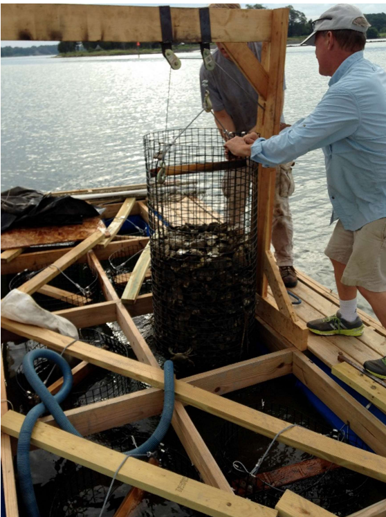
The hoist in action... yep, should have made it a little taller. We used a self-locking winch I had laying around... I highly recommend that style as ratchet could "get away from you". The span bar is a 2x6" untreated. Also, we overbuilt, no need to make this "a double" we should have just slid a single pulley to whichever side we wanted to lift up.
