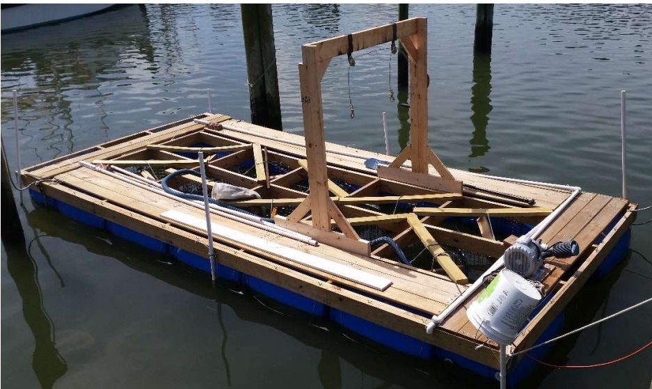
Hoist on barge... note that the tarp has been removed. Oysters are growing in the cages... an ice eater circulating water probably would have sped the growth some. Instead of crane I had originally worked on a mechanism to lower the bottom of the cage down with a long threaded rod. I should have just started with a hoist like this, plus it lets one check the set rate.
