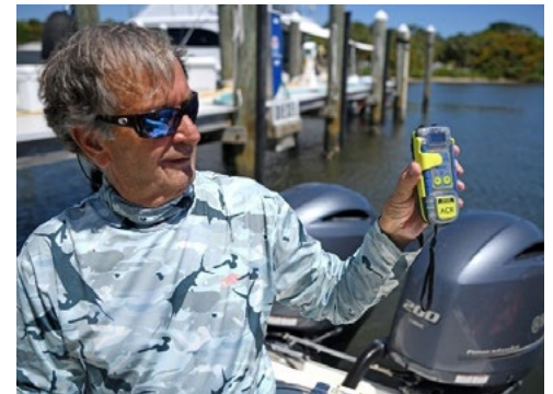
The BoatUS Foundation offers GPS-enabled, 406-MHz Personal Locator Beacons for rent, as well as EPIRBs.
