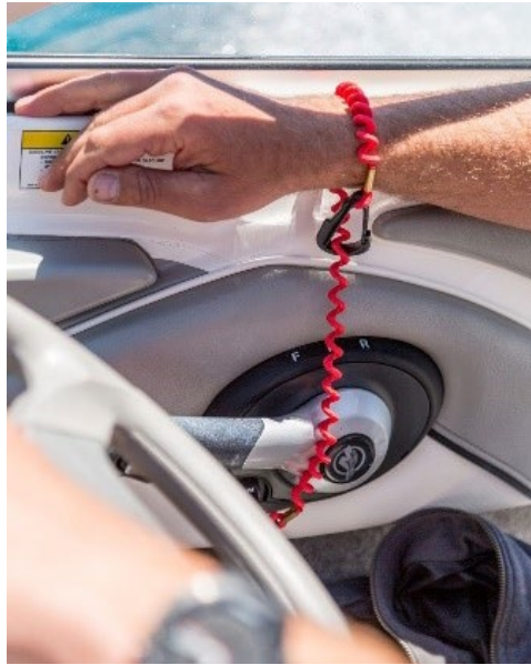
Engine cutoff switches (ECOS) are often activated by a lanyard connected to the operator that, when pulled, stops the boat’s engine. (Credit: National Safe Boating Council)
